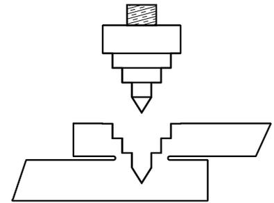
Figure 3. Custom Step Tip Design
